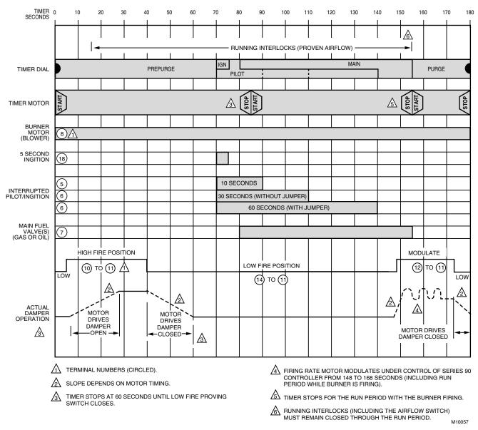
Fig. 12. Timer sequence for R4140G1171, R4140G1122 and R4140G1114 Programmers.
